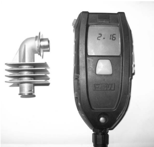
Fig. 2 New type of pre-cooler, display of IC-Air software version
